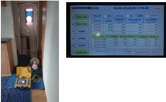
Photo 3.1: Airtightness measurement (C-value Measurement) Left: Measurement scene Right: Measurement result monitor
