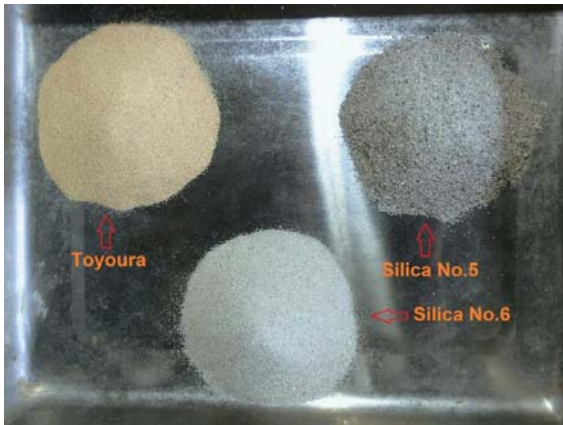
Figure 10. Actual images of the three types of sand used in this study
