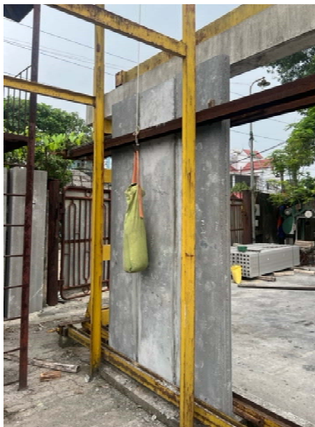
Figure 7. Experiment to evaluate the impact resistance of precast concrete hollow wall panels using thermoelectric ash and slag
