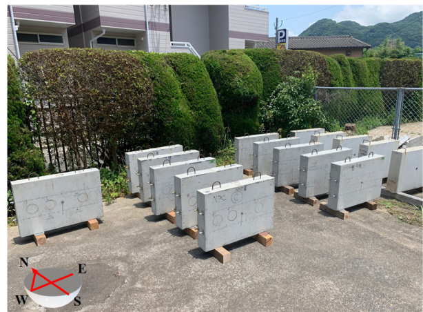
Photo 1. Wall specimens under exposure test
