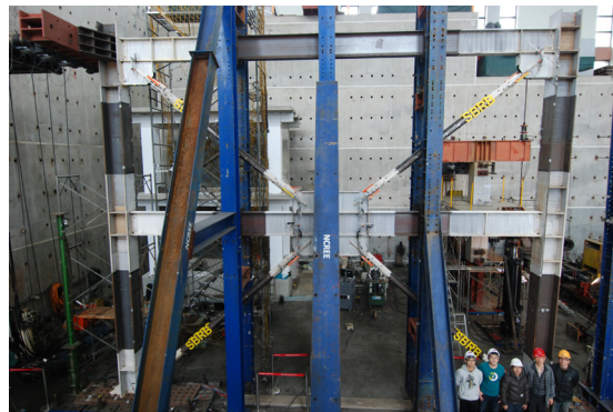
(b) Phase 1 test (1.6% second floor drift)
