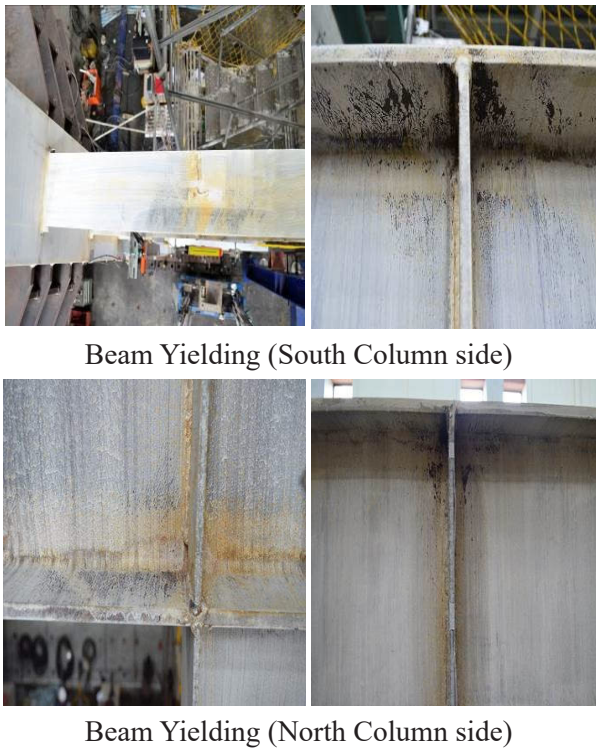
Figure 3. Observed performance in Phase 1 test (1.6% second floor drift).
