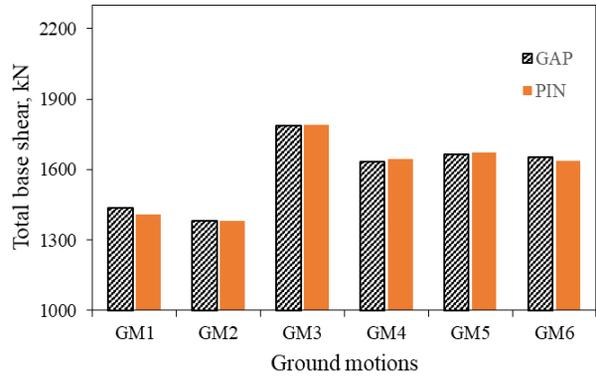
Figure 8. Total base shear ( $S_a = 0.2$  g)
