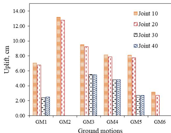
Figure 6. Maximum uplift of Gap model
