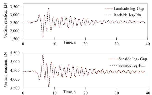
**Figure 12. Vertical reaction of Imperial Valley-06, 1979 earthquake ( $S_a = 0.2 g$ )**
