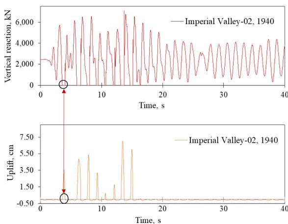
Figure 5. Uplift and reaction of landside leg – Joint 10
