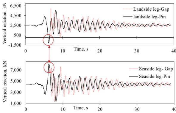
**Figure 11. Vertical reaction of Imperial Valley-06, 1979 earthquake ( $S_a = 0.8 g$ )**
