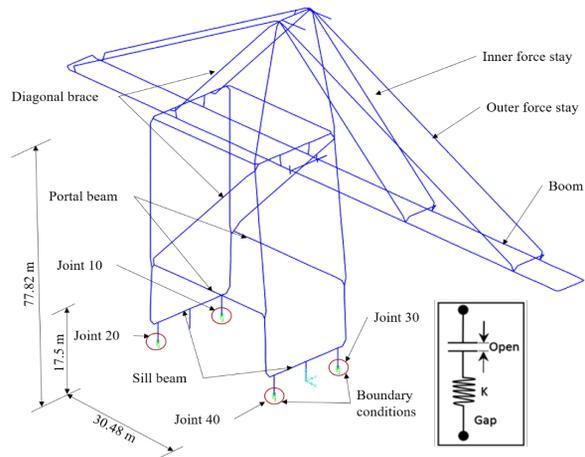
**Figure 1. 3D model of container crane**
