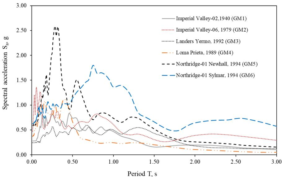
**Figure 2. Original response spectral accelerations**
