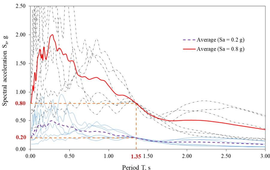
**Figure 3. Scaled response spectrum at the fundamental period**
