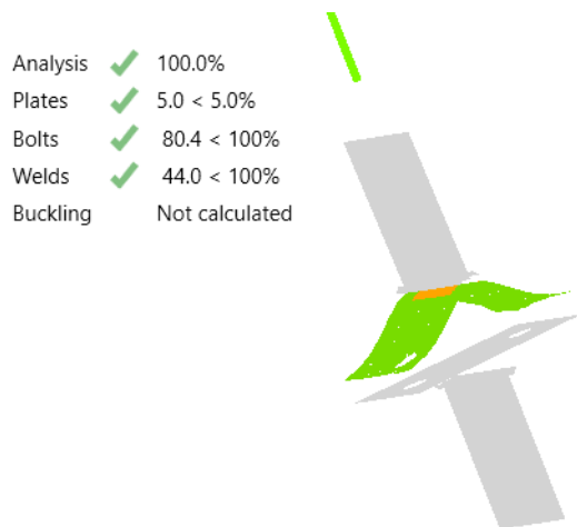
Figure 16. Failure mode 2 in CBFEM
