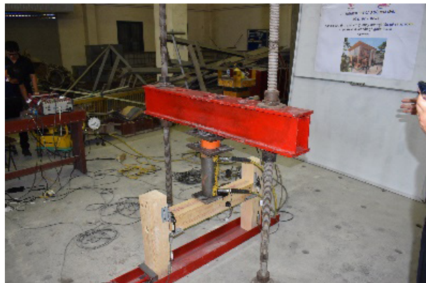
Figure 4. Shear failure test of metal joint by IBST
