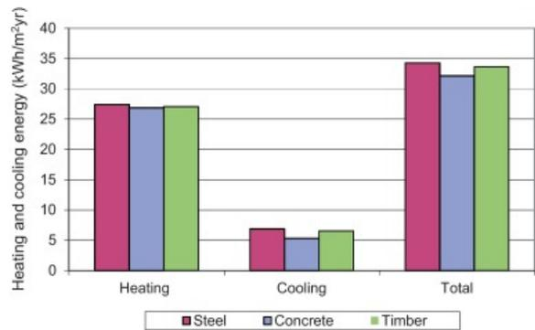
Figure 5. Annual operational energy requirements of the three construction types, per m<sup>2</sup> of floor area.
