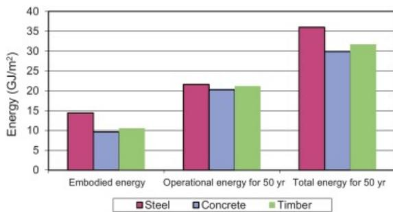
**Figure 6. Life cycle energy requirements of the three construction types over 50 years.**
