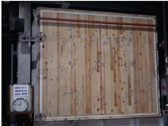
Figure 15. Non-burned surface after test
