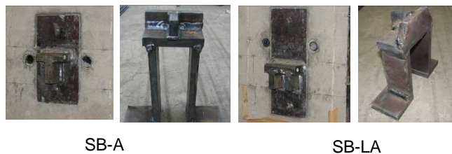
Figure 3. Shear bracket and U-shaped steel box
