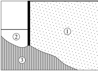
Zone 1 – Vertical stresses remain while horizontal stresses gradually reduce when excavating
