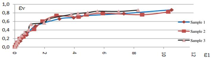
**Figure 2.20. Interrelated diagram between volume deformations and axial deformations**
