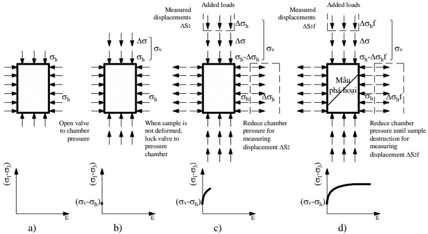
**Figure 2.4. Testing progress scheme**
