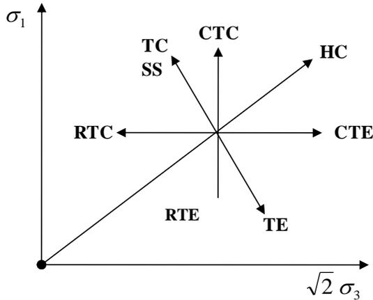
**Figure 1.6. Reflected diagram for different stress lines on three-direction plan**
