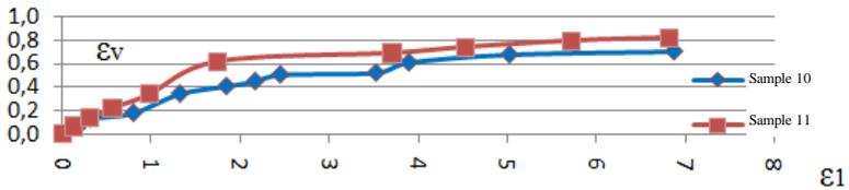
**Figure 2.31. Interrelated diagram between volume deformations and axial deformations**
