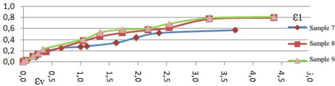
**Figure 2.26. Interrelated diagram between volume deformations and axial deformations**
