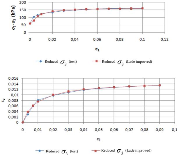
**Figure 3.21. Compare on calculation results and stress-deformation relationship results for reduced tri-axial compression tests  $\sigma_3$**
