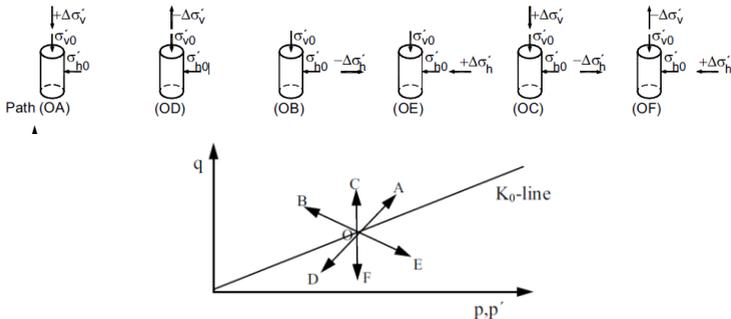
**Figure 1.1. Different stress schemes on one excavated pits**
