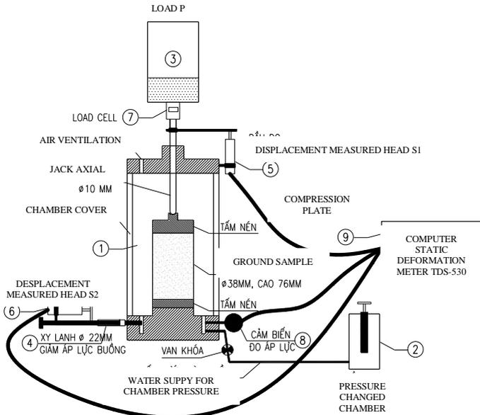
**Figure 2.5. Machine diagram for horizontal stress-reduced experiments**
