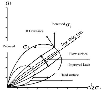
**Figure 3.13. Improved plastic flow surface Lade**
