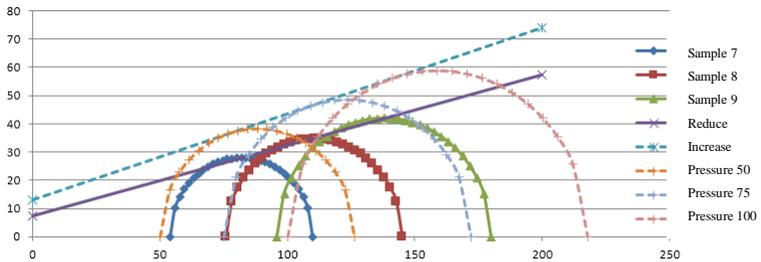
**Figure 2.32. Mohr circle diagram of horizontal stress tests and compare with conventional tri-axial tests**
