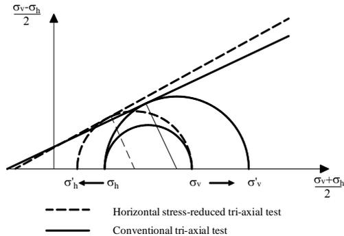
**Figure 2.1. Destructive boundary diagram Mohr - Coulomb**
