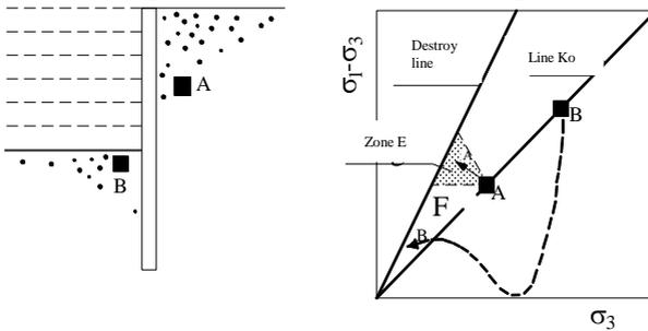
**Figure 1.4. Stress line on excavated pits**
