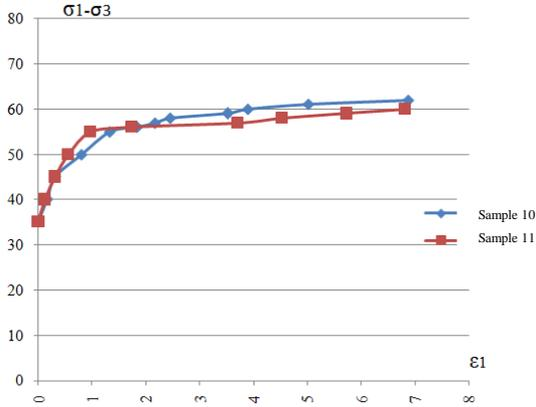
**Figure 2.30. Interrelated diagram between stress deflections and axial deformations**
