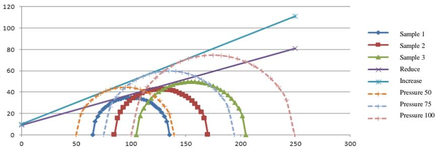
**Figure 2.21. Mohr circle diagram of horizontal stress tests and compare with conventional tri-axial tests**
