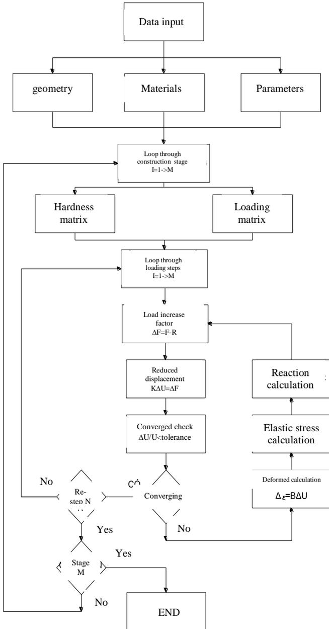
**Figure 3.24. Block and loop-solving diagram of LadeDeep software**
