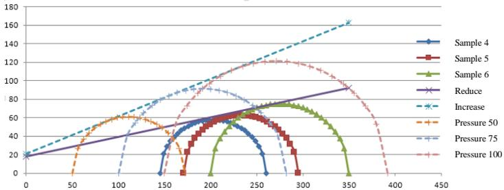
**Figure 2.27. Mohr circle diagram of horizontal stress tests and compare with conventional tri-axial tests**
