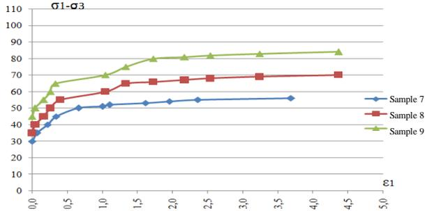
**Figure 2.25. Interrelated diagram between stress deflections and axial deformations**
