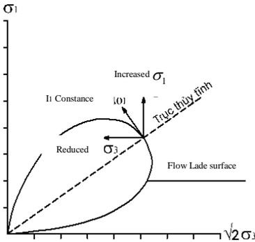
**Figure 3.12. Stress path of tri-axial compression test and flowing surface Lade**
